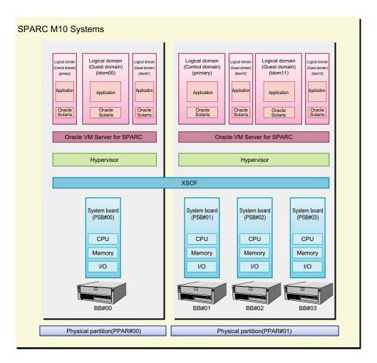
The main firmware and software used in SPARC M10 Systems are as follows.
